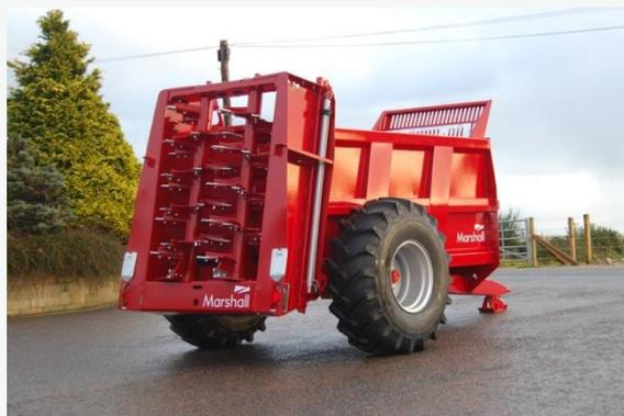
**ALWAYS** close the slurry door after spreading, this firstly protects the ram and avoids unnecessary stress on the door slides when travelling.
