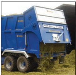
Hyd Grain Door c/w Silage Attachment
