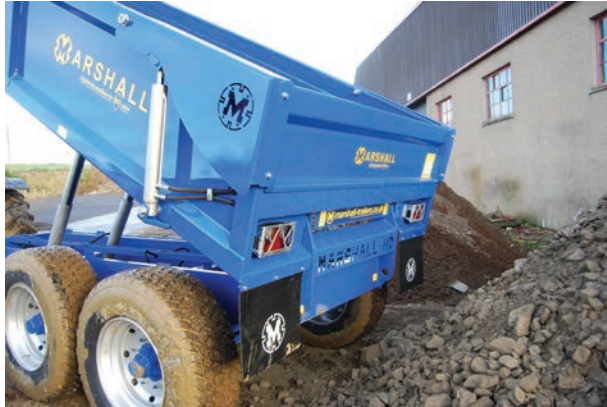
Dealer Fit Hydraulic Door & Elevated Tipping Points
