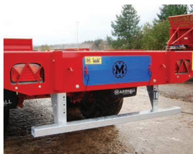
Left: Recessed Lights, Rear Crash Barrier and Toolbox Right: 5/8" Diameter Rope Hooks & Integrated Strap Points
