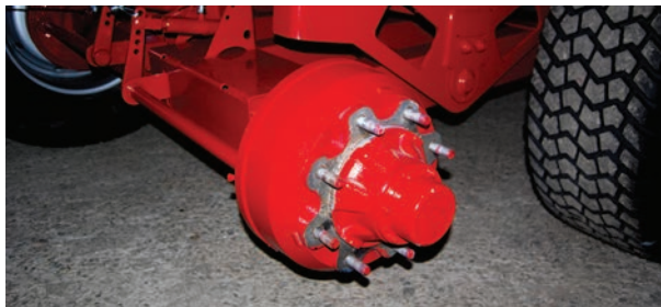
Rocker Tandem Suspension
