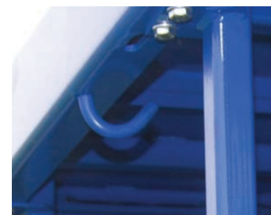
Left: Recessed Lights, Rear Crash Barrier and Toolbox Right: 5/8" Diameter Rope Hooks & Integrated Strap Points
